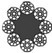
8 x 19S+ Fibre core (CFN)
